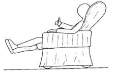
The user must always be positioned within the wheel base of the chair. A posture belt may be necessary to achieve this at all times.
